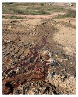
Leachate seep at Cell 6 NW slope (inactive area)
